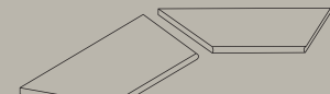
ANGOLARE INTERNO BORDO TORO INT. BULLNOSE EDGE CORNER ▲ 60x120 (24"x48") RT 20mm ▲ 30x120 (12"x48") RT 20mm ▲ 30x60 (12"x24") RT 20mm
