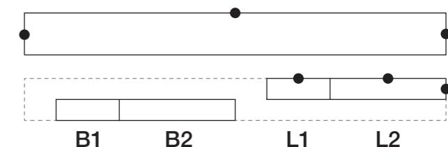
STRIP The strip can be cut into the side pieces L1 and L2 and the skirting elements B1 and B2.
